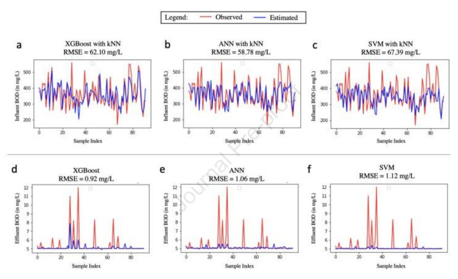
**Figure 5** Visual comparison and RMSE (mg/L) of (a) *BOD<sub>inf</sub>* estimated by XGBoost; (b) *BOD<sub>inf</sub>* estimated by ANN with kNN; (c) *BOD<sub>eff</sub>* estimated by SVM with kNN; (d) *BOD<sub>eff</sub>* estimated by XGBoost; (e) *BOD<sub>eff</sub>* estimated by ANN with kNN; and (e) *BOD<sub>eff</sub>* estimated by SVM with kNN, modelled using the Hong Kong dataset.
