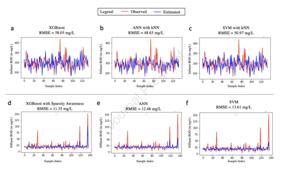
**Figure 4** Visual comparison and RMSE (mg/L) of (a) *BOD<sub>inf</sub>* estimated by XGBoost; (b) *BOD<sub>inf</sub>* estimated by ANN with kNN; (c) *BOD<sub>eff</sub>* estimated by SVM with kNN; (d) *BOD<sub>eff</sub>* estimated by XGBoost; (e) *BOD<sub>eff</sub>* estimated by ANN with kNN; and (e) *BOD<sub>eff</sub>* estimated by SVM with kNN, modeled using the UCI Machine Learning Repository dataset.
