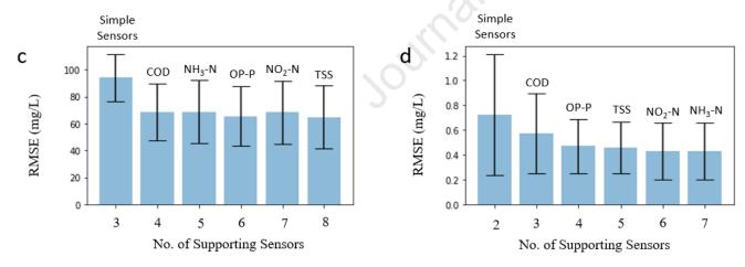
Figure 3 Change in RMSE (mg/L) supporting sensors are incrementally added to the soft sensor for (a, c) influent BOD and (b, d) effluent BOD.
