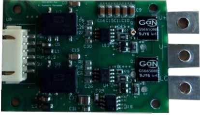
Fig. 8: The implemented GaN based half-bridge inverter module
