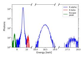
FIG. 2. The x-ray source spectrum as recorded with the SLcam. The gallium K-alpha peak (9.25 keV) along with the double pileup (18.5 keV) and triple pileup peaks (27.75 keV) are shown in blue. The K-alpha escape peak in silicon (7.51 keV) is shown in green and the K-beta (10.26 keV) is shown in red.
