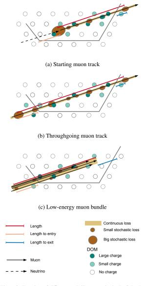
Figure 3: Top view of different track-like events in the IceCube detector, showing quasi-continuous and stochastic energy losses as well as the definition of three useful track length variables. Figure adapted from [14].
