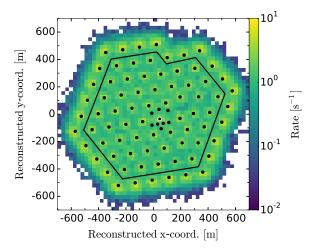
(a) Top view of the IceCube detector where string positions are shown as black dots. The polygon shape represents the containment criterion for the reconstructed interaction vertices (see also Fig. 1).
