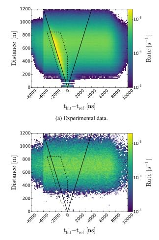
(b) Simulated, truly down-going, muon neutrinos interacting inside the volume defined by the dotted polygon in Fig. 1 and  $z \le 300$  m.
