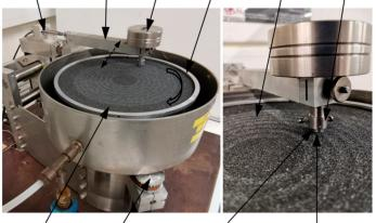
Abrasive paper Motor drive Specimen Multi-asperity contact
