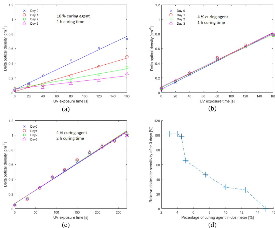
**Figure 1.** Stability of the dose response for (a) FlexyDos3D 10 % mixture and (b) FlexyDos3D 4 % mixture cured for 1 hour at 60 °C, and (c) FlexyDos3D 4 % mixture cured for 2 hours at 60 °C. Note that (c) was investigated for a longer exposure time and with more sample points. (d) Sensitivity of dosimeters with different curing agent concentrations after 3 days relative to the first measurement.
