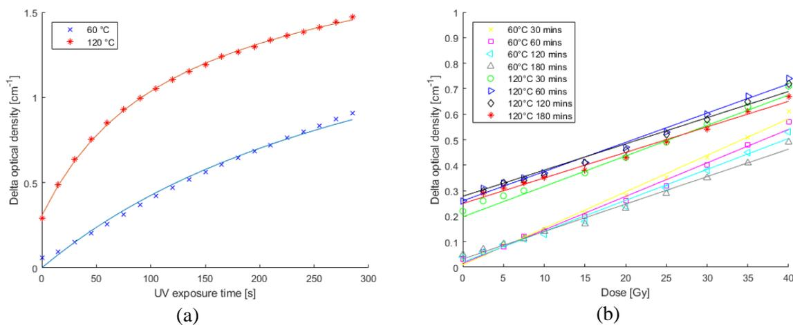
**Figure 2.** Optical density difference between 630 nm and 480 nm versus UV exposure time for two FlexyDos3D 4% C samples cured at different temperatures for 60 minutes (a). Optical density difference between 630 nm and 480 nm versus radiation dose for different curing temperatures and times (b). The use of the difference in optical densities at the two wavelengths can compensate for some of the artefacts in the cuvettes caused by the contraction of the dosimeter after cooling.
