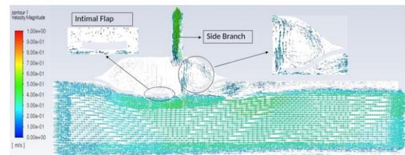
Figure 1. Velocity vectors at  $t = 0.24375$  s during the deceleration phase of the cardiac cycle.
