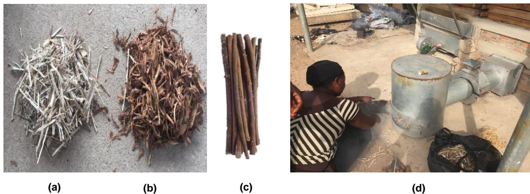
Fig. 3.3: Materials for generating smoke (a=Sugarcane bagasse; b= coconut husk; c= A. indica sticks) and smoke-generation for indirect smoke-flavouring on the FTT (d)
