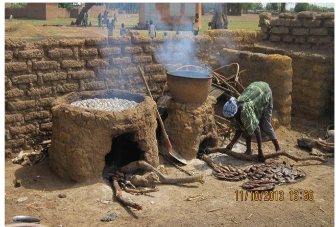
d) Cylindrical mud oven (Fante oven, left), and a traditional mud oven (daging) in Burkina Faso (right) [Source: Mindjimba et al., 2019]
