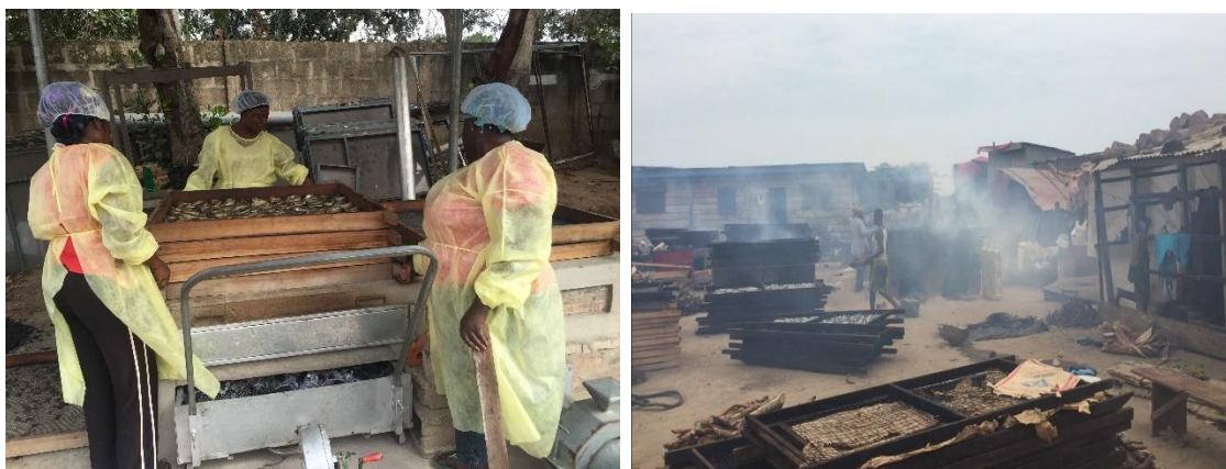
Fig. 7.1: Comparison of smoke exposure during the use of the FTT (left) and the Chorkor smoker (right)
