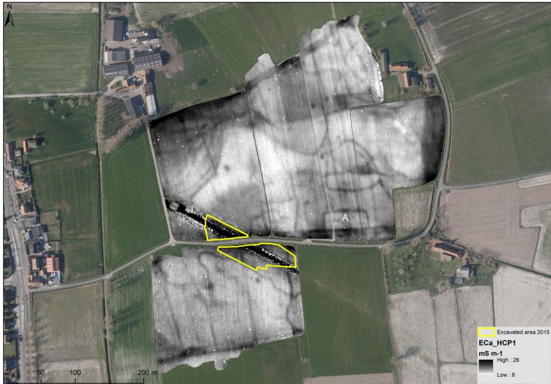
Figure 33: Eca-HCP1 electrical conductivity plot of EMI survey at Brugge-Dudzele-Kruisabelestraat.
