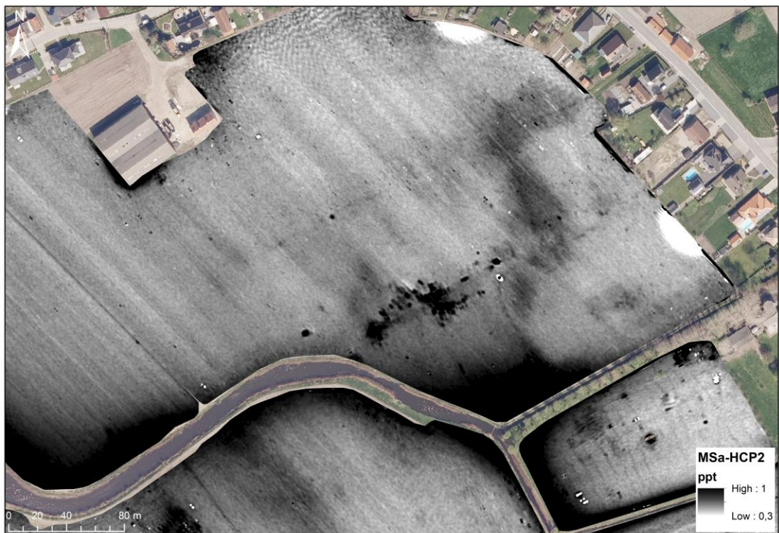
Figure 60: ECa-HCP1 and MSa-HCP2 detail showing the interpreted settlement core at Nieuw-Roeselare. See Figure 64 for interpretation.
