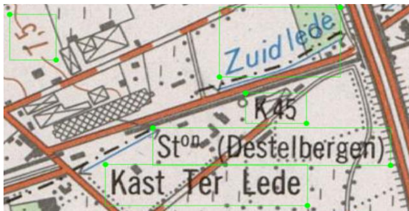
Figure 1: Example of some text labels from one of the topographic maps. These text labels can come in different colors, orientations, and sizes, complicating automated processing techniques.
