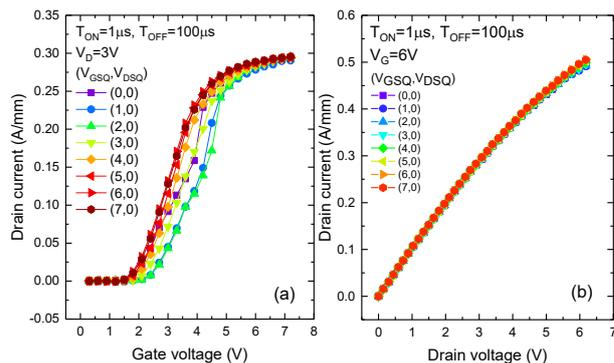
Fig. 2. Double pulse measurements showing the drain current versus (a) gate voltage at  $V_D = 3 \text{ V}$  and (b) drain voltage at  $V_G = 6 \text{ V}$ . No degradation in ON-resistance is observed, indicating that the trapping phenomena are concentrated under the gate region. The stress and measurement pulse last 100 and 1  $\mu$ s, respectively.
