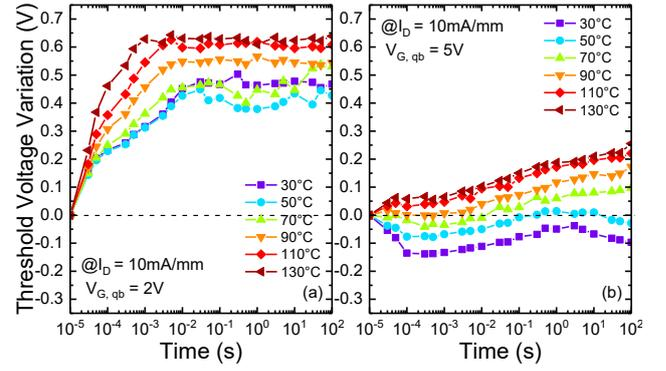
Fig. 4. Experimental threshold voltage variation versus stress time at different temperatures for (a)  $V_G = 2$  V and (b)  $V_G = 5$  V.
