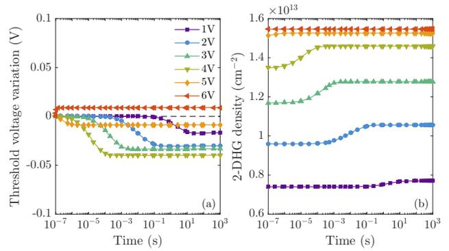
Fig. 7. (a) Simulated threshold voltage variation versus stress time without acceptor traps at the AlGa<sub>n</sub>/Ga<sub>n</sub> interface. (b) Hole density in the 2-DHG versus stress time for different ON-state stress voltages.
