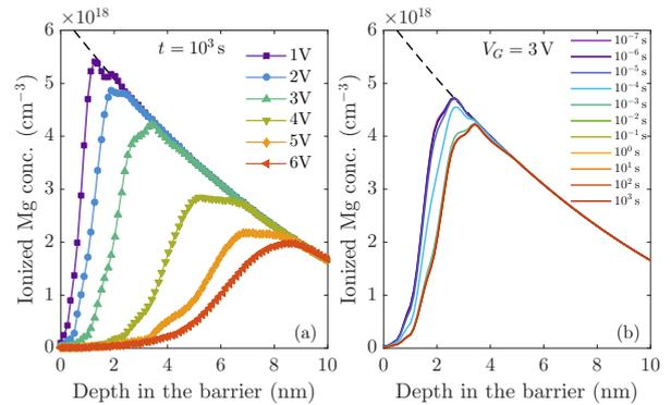
Fig. 8. Simulated ionized Mg charge density versus depth in the barrier, relative to the  $p$ -Ga<sub>n</sub>/AlGa<sub>n</sub> interface, (a) for different gate bias at  $t = 10^3$  s, and (b) for different stress time at  $V_G = 3$  V. The Mg out-diffusion tail is represented in black dashed line.
