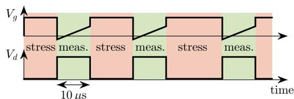
Fig. 1. Schematic representation of the gate and drain voltage during the threshold voltage transient measurement. The ‘stress’ and ‘measurement’ phase are shown in red and green, respectively.
