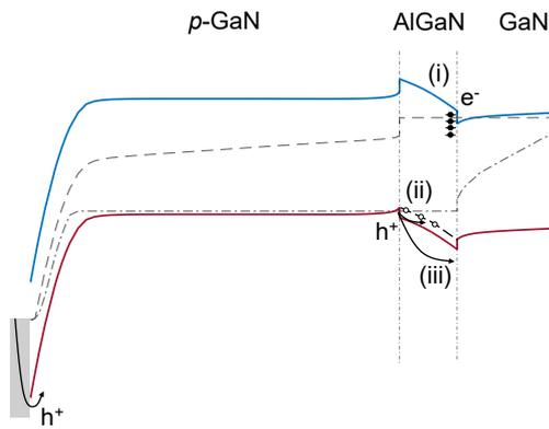
Fig. 9. Energy band diagram of the Schottky metal/*p*-GaN/AlGaN/GaN gate stack at  $V_G = 6\text{ V}$  with three different threshold voltage variation mechanisms.
