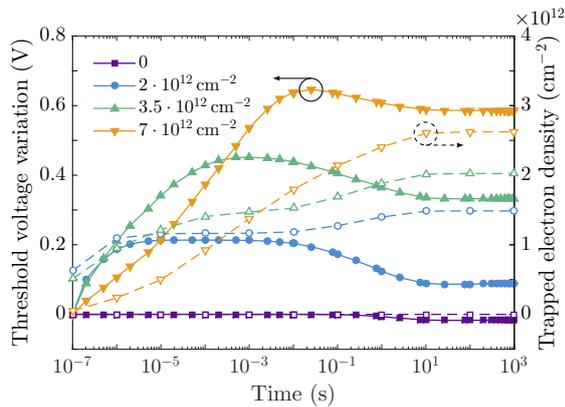
Fig. 6. Left axis: threshold voltage variation versus stress time at  $V_G = 1$  V for increasing interface trap density at the AlGa<sub>n</sub>/Ga<sub>n</sub> interface. These states are uniformly distributed between 0.05 and 0.65 eV below the conduction band. Right axis: interface trapped electron density at the AlGa<sub>n</sub>/Ga<sub>n</sub> interface versus stress time.
