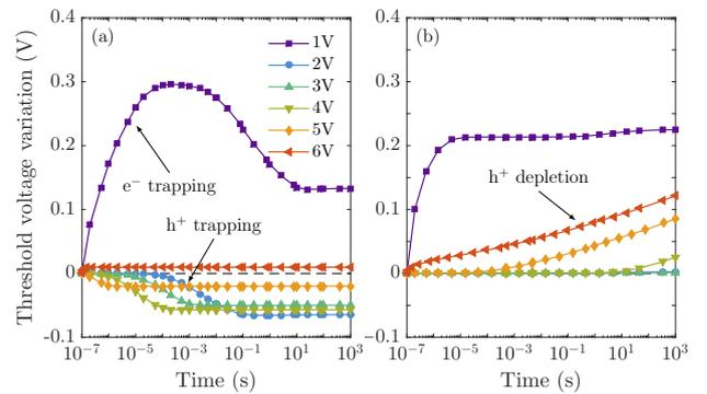
Fig. 5. Threshold voltage variation extracted from TCAD simulations at room temperature in the case of (a) low and (b) high  $p$ - $i$ - $n$  diode leakage level. Both cases are simulated with a highly conducting Schottky gate.
