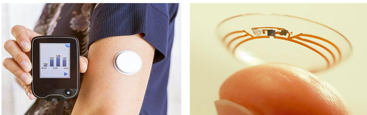
Figure 7: Left panel: the FreeStyle Libre, a sensor that continuously measures glucose in ISF. Right panel: Smart Contact Lens developed by Google for glucose monitoring 60-61 .
