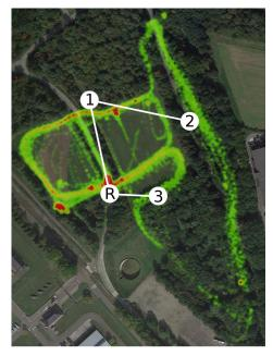
Fig. 11: Heatmap of all location observations measured during the cyclo-cross training. It shows the data measured during the active periods of all riders and the location of the three static CONAMO devices (1, 2 and 3) and the sink node (R).
