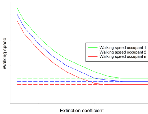
Figure V.8: Schematic representation of the fractional/variable minimum speed interpretation.
