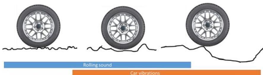
Figure 2: Relationship between rolling noise and car vibrations to the road profile.
