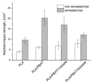
Figure 2. The notched impact strength of samples before and after annealing
