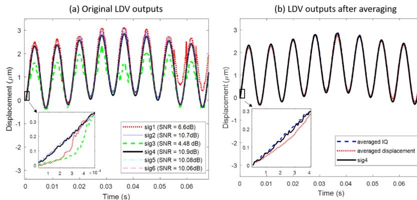
Fig. 2. The averaging effect of six signals: (a) six demodulated signals in which channel 1 and channel 3 show strong deviations due to speckle. (b) Comparisons of the best demodulated signal (channel 4), IQ-averaged signals and displacement-averaged signals.
