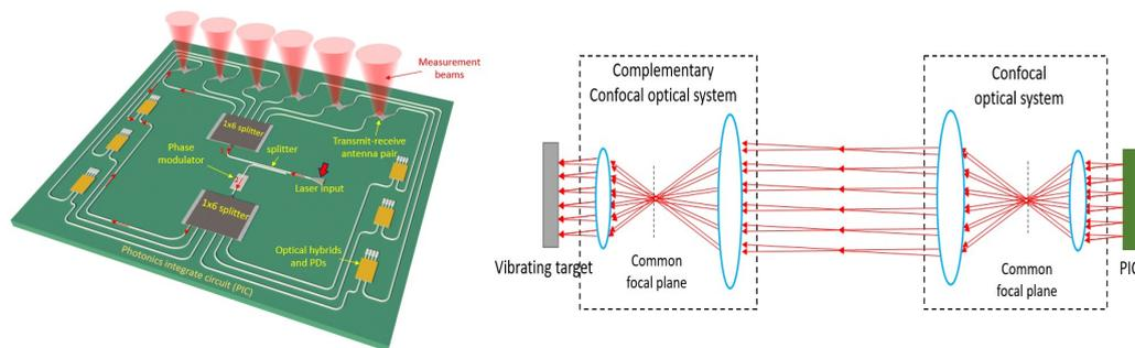
Fig. 1. (a) Schematic show of the external confocal optical system, the six-beam LDV on an SOI-based photonic integrate circuit (PIC). (b) Schematic show of the system used in the de-speckle experiments. The dimensions of the lenses in the drawing are exaggerated to make the design easier to understand.
