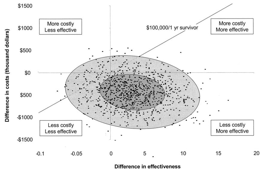
Fig 13 – Visualisation of Monte Carlo based PSA (1000 simulations) with the example indicating that the new intervention is most probably less costly and more effective than the comparator. Ellipses represent 50% and 95% confidence intervals. Illustration from D. Angus et al. *Pediatrics*, 6/12/2003[143]
