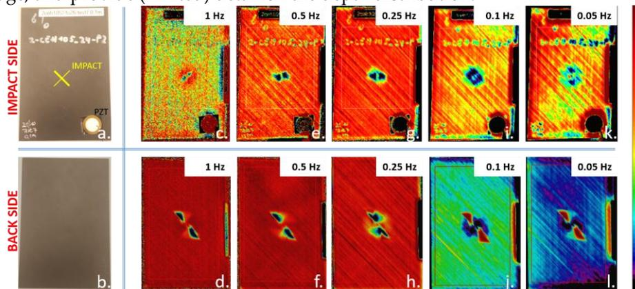
Figure 7: IRT in reflection of impact side (top row) and backside (bottom row) of  $CFRP_{BVID}$ : (a-b) photograph; phase images at (c-d) 1 Hz, (e-f) 0.5 Hz, (g-h) 0.25 Hz, (i-j) 0.1 Hz and (k-l) 0.05 Hz.
