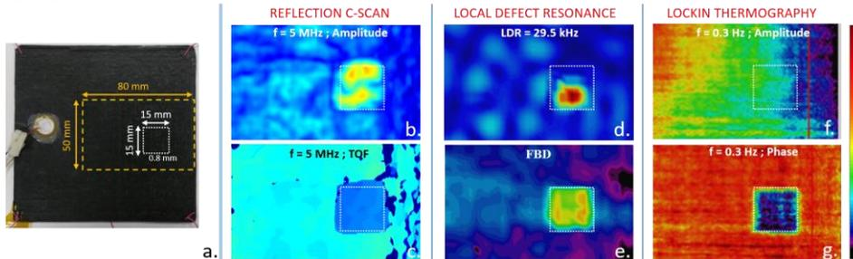
Figure 4: Results for CFRP<sub>INSERT</sub>: (a) photograph of inspected area. Ultrasonic C-scan at 5 MHz: (b) reflected amplitude and (c) TOF. Vibrational testing: (d) LDR at 29.5 kHz and (e) frequency band data FBD over 5–100 kHz. Lock-in thermography at 0.3 Hz: (f) amplitude and (g) phase image.
