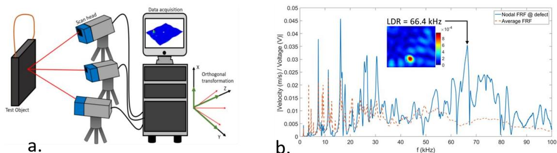
Figure 2: (a) Principle of 3D scanning laser Doppler vibrometry and (b) FRF of a [45/0/-45/90]<sub>3S</sub> CFRP sample with a flat bottom hole (diameter of 10 mm).
