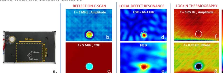
Figure 3: Results for CFRP<sub>FBH</sub> : (a) photograph of inspected area. Ultrasonic C-scan at 5 MHz: (b) reflected amplitude and (c) TOF. Vibrational testing: (d) LDR at 66.4 kHz and (e) frequency band data FBD over 50-100 kHz. Lock-in thermography at 0.05 Hz: (f) amplitude and (g) phase image.
