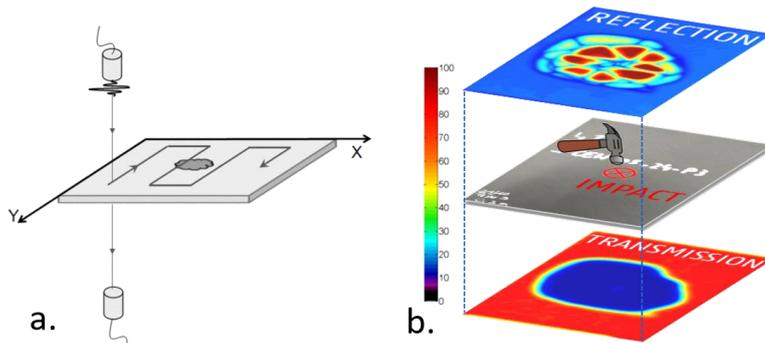
Figure 1: (a) Principle of C-scan and (b) ultrasonic C-scan in reflection (top) and transmission (bottom) for an impacted  $[45/0/-45/90]_{3s}$  CFRP (middle) with impact energy 18.5 J. The color scale indicates the amplitude level.
