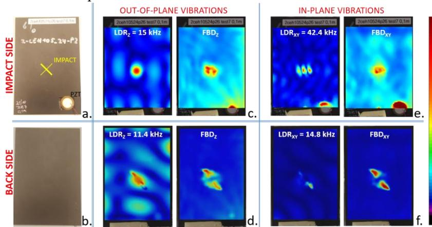
Figure 6: Results of impact side (top row) and backside (bottom row) of  $CFRP_{BVID}$ : (a-b) photograph of sample, (c-d) out-of-plane  $LDR_z$  and frequency band data  $FBD_z$  over 2-100 kHz and (e-f) in-plane  $LDR_{xy}$  and frequency band data  $FBD_{xy}$  over 2-100 kHz.
