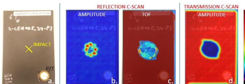
Figure 5: (a) photograph of CFRP<sub>BVID</sub>, (b) amplitude reflection C-scan, (c) TOF reflection C-scan and (d) amplitude transmission C-scan.
