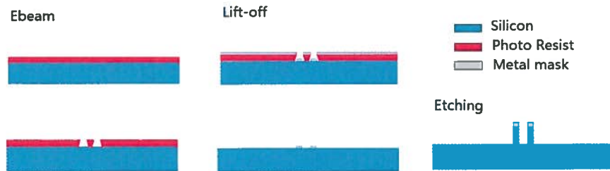
Figure 4: fabrication of master mold
