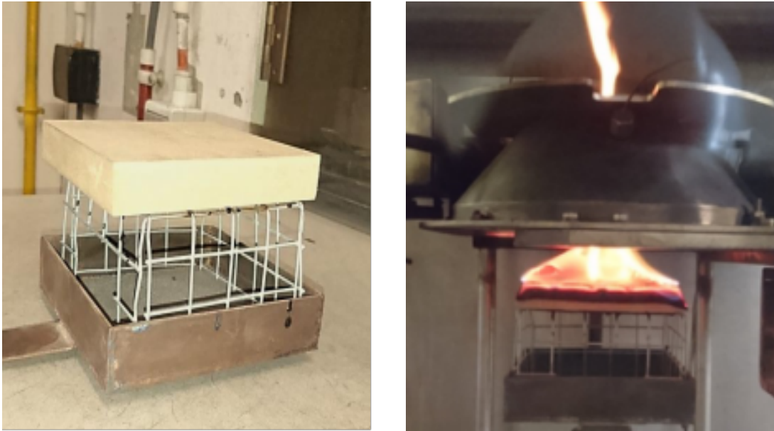
Figure 3.20: The MDF sample in the cone calorimeter test.
