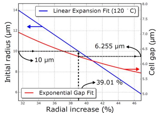
**Figure 1: Initial spacer radius and resulting cell gap as a function of radial spacer increase during bonding**
