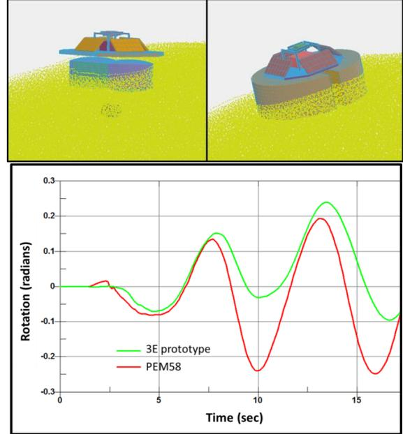
Figure 3: Comparison between the rotations of 3E and PEM58 buoys
