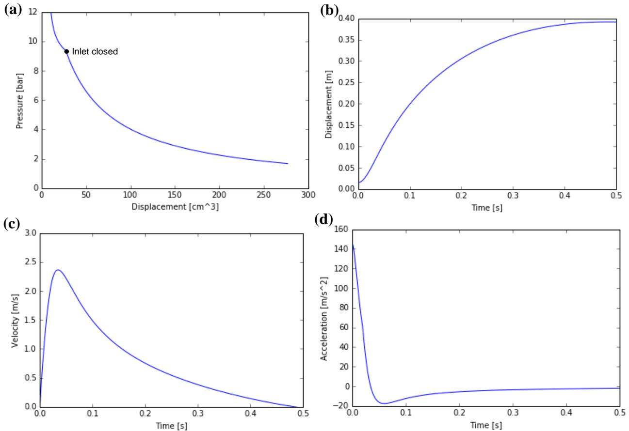
Fig. 4. a) *p-V* diagram, b) piston displacement, c) piston velocity, d) piston acceleration in function of time for the working fluid cyclopentane.
