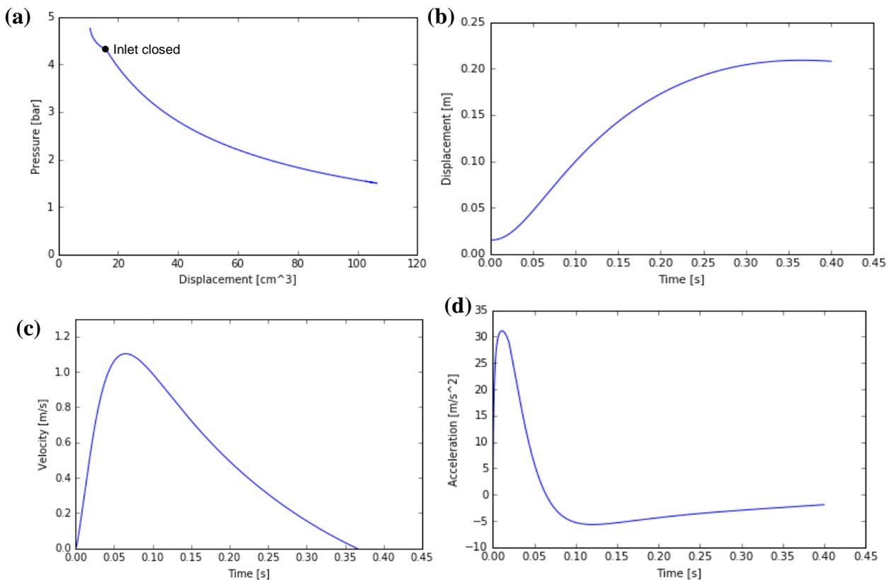
Fig. 2. a) p-V diagram, b) piston displacement, c) piston velocity, d) piston acceleration in function of time for the working fluid water.
