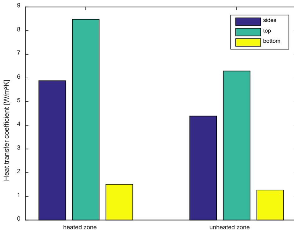
*Fig. 1. Values for the heat transfer coefficient on the different surfaces.*
