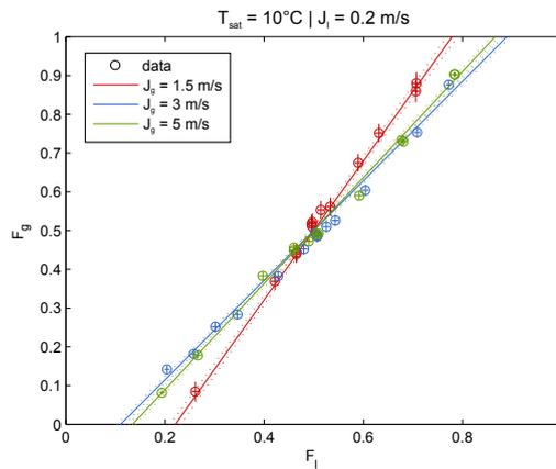
Figure 5: The vapour mass fraction as function of the liquid mass fraction for R32 divided over an impacting T-junction ( $T_{sat} = 10\text{ }^{\circ}\text{C}$ ;  $J_l = 0.2\text{ m/s}$ ).
