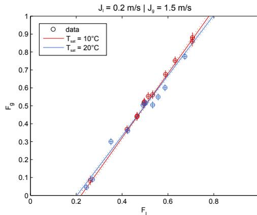
Figure 6: The vapour mass fraction as function of the liquid mass fraction for R32 divided over an impacting T-junction ( $J_g = 1.5\text{ m/s}$ ;  $J_l = 0.2\text{ m/s}$ ).
