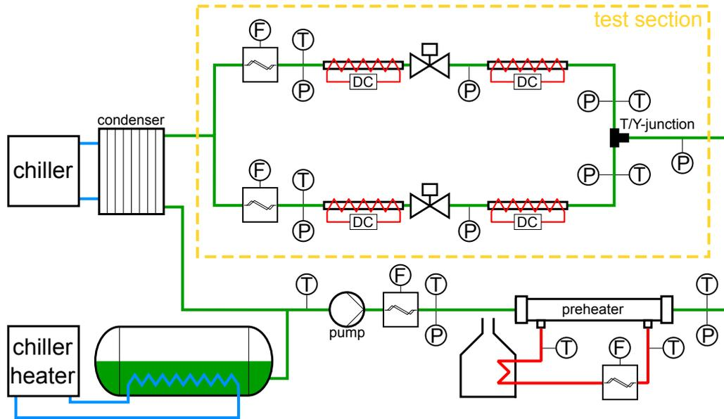
Figure 2: A schematic representation of the experimental setup.
