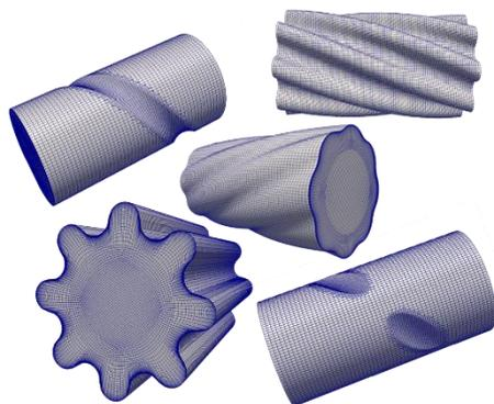
Figure 2: Structured meshes of complex 3D reactor geometries.
