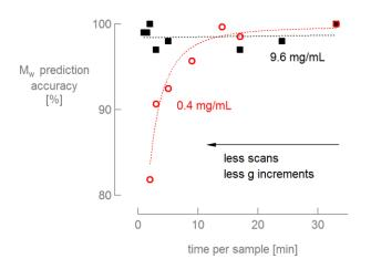
*Figure* 8. Influence of DOSY measurement time, as a result of the applied number of scans and field strength gradient (g) increments, on the accuracy of weight-based molecular weight ( $M_w$ ) prediction for high ( $\blacksquare$ , 9.6 mg mL<sup>-1</sup>) and low ( $\bullet$ , 0.4 mg mL<sup>-1</sup>) concentration PEF samples. The lines are to guide the eye.
