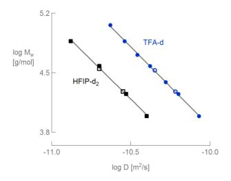
*Figure 10.* Comparison of PET calibrations in more viscous HFIP- $d_2$  (**■**) and TFA-d (**●**), and the resulting M<sub>w</sub> predictions for two PEF samples in HFIP- $d_2$  (**□**) and TFA-d (**○**). Predicted M<sub>w</sub> were 18,970 g mol<sup>-1</sup> and 35,290 g mol<sup>-1</sup> (**□**) compared with MALS values 19,150 g mol<sup>-1</sup> and 33,850 g mol<sup>-1</sup> (**○**), respectively.
