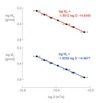
*Figure 3.* DOSY calibration curve of PET standards ( $M_w = 9,870 \text{ g mol}^{-1} - 115,000 \text{ g mol}^{-1}$ ) in TFA-*d* derived from fully (5%) attenuated aromatic proton signal decay curves. Error bars were calculated using t-statistics on the variance of >3 repetitions per sample.
