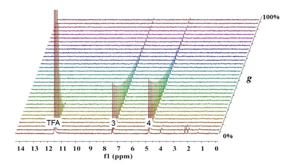
*Figure 2*. Stacked increments of <sup>1</sup>H NMR spectra of PEF (7.46 ppm = 3 = Furan, 4.88 ppm = 4 = Ethylene Glycol) in TFA-*d* (11.7 ppm = TFA) with increasing gradient strength *g*.
