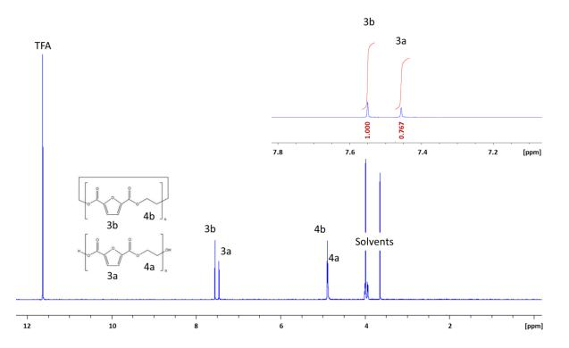
*Figure 5.* <sup>1</sup>H NMR of a PEF sample taken from the ring-opening polymerization reactor. The separated chemical shifts of the furanic unit and the Ethylene Glycol incorporated in the PEF polymer (3a, 4a) and the cyclic monomer (3b, 4b) respectively, can be used for individual molecular weight analysis.
