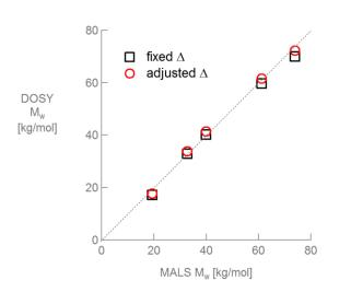
*Figure 9.* PEF samples analyzed with PET calibrations derived from data obtained using fixed and adjusted diffusion times  $\Delta$ .
