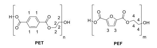
Figure 1. Molecular structures of PET (left) and PEF (right)
