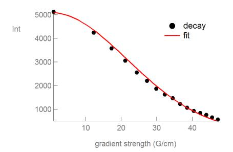
*Figure S2.* Exemplary signal intensity (Int) decay curve of furan protons (chemical shift = 7.46 ppm) derived from DOSY on a PEF sample (•, MALS  $M_w = 39910$  g/mol) using diffusion time  $\Delta = 600$  ms. The data was fitted (—) with the Stejskal-Tanner equation (equation 1) to derive a diffusion coefficient  $D = 3.982 \cdot 10^{-11}$ , which using the PET calibration (Figure 3) resulted in an  $M_w = 41480$  g/mol.
