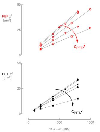
*Figure* 7. Evaluation of unhindered Gaussian diffusion conditions via mean square displacement  $z^2$  analysis. Tested concentrations were 0.4, 3.1, 9.5, 20.8, 35.5 mg mL<sup>-1</sup> for PEF and 0.4, 0.7, 4.3, 8.7, 30.4 mg mL<sup>-1</sup> for PET.
