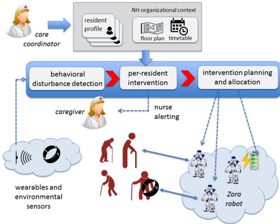
Figure 1. Behavioral disturbances are detected by combining sensor and wearable data with context information. The platform alerts a caregiver or creates a companion robot intervention task. Tasks are scheduled over a pool of robots, taking into account their current position and battery level.
