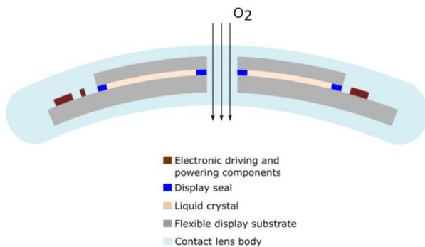
**Fig 2. Cross section of the smart contact lens illustrating how a central hole in the display can allow extra oxygen transfer to the eye.**
