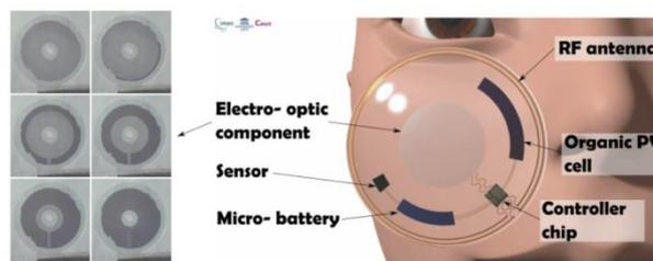
**Fig 1. LC display with concentric rings (left); smart contact lens containing a LC display, powering and steering components (right).**
