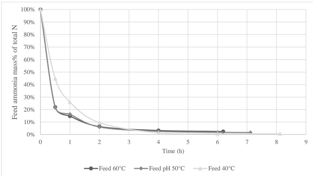
**Figure 4:** Feed mass percentage of total ammonia versus total time of the membrane distillation experiment. Urine of batch Hydro-01 was used, with a feed pH of 10.5. The membrane used in this series of experiments came from a single sheet of S02 membrane.
