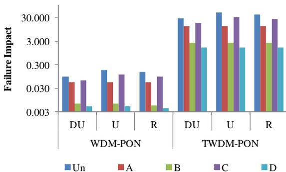
Fig. 5: Failure impact (FI) of different schemes for WDM- and TWDM-PON
