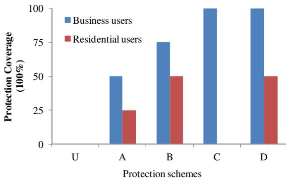
Fig. 3: Protection coverage of different schemes for WDM- and TWDM-PON
