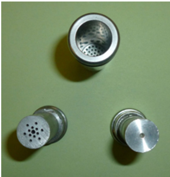
Fig. 5 Traditional (right) and modified (left) perforated plunger according to Teipel and Winter [25]
