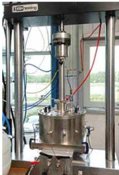
Figure 4: Corrosion fatigue crack growth rate equipment [10]
