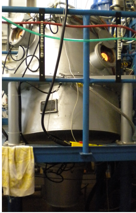
Figure I.1: Picture of the plasma gasification reactor at the IPP during operation
