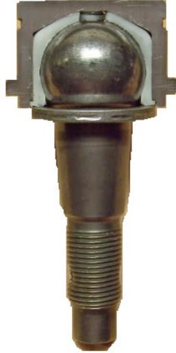
Figure 2: Cutaway section of a ball joint
