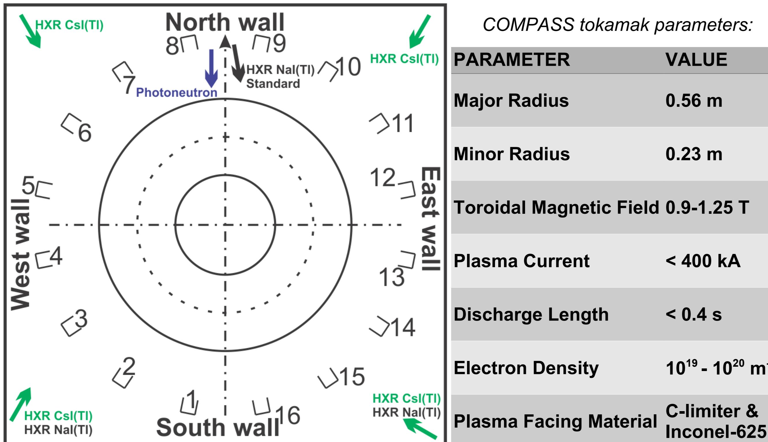
Experimental setup of diagnostics used for RE loss detection during the 2<sup>nd</sup> COMPASS RE campaign.
