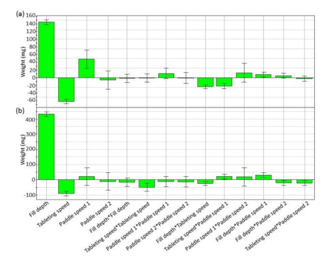
Figure 2: Effect plot of tablet weight. (a) MCC, (b) DCP.
