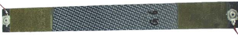
Figure 4 Specimen prepared with rivets for electrical resistance measurement.
