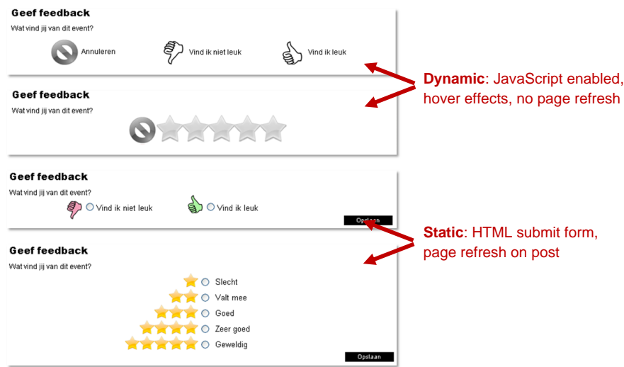
Figure 3.2: Four explicit feedback systems (5-star scales and thumbs up/down) as commonly found online. User interface text in Dutch because they were integrated in a Belgian website.
