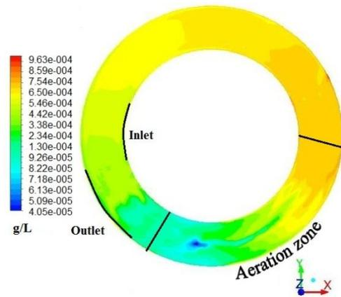
Figure 8 Ammonium conc. contour plot at 3m depth
