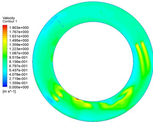
Figure 4 Velocity contour plot at 3m depth
