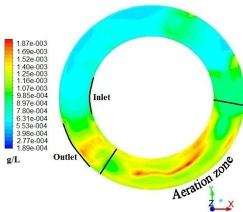
Figure 7 Oxygen conc. contour plot at 3m depth
