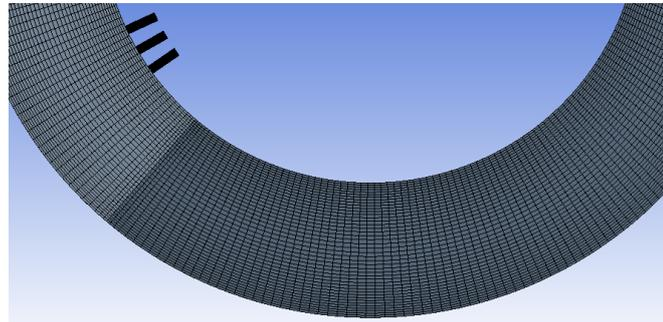
**Figure 2** Top view of the reactor mesh
