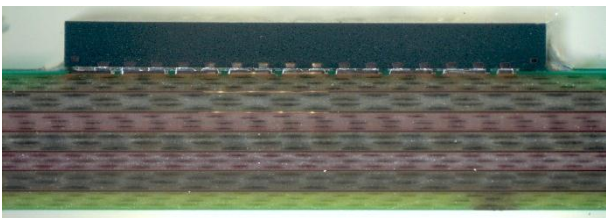
Figure 6: Side view of the QFN64 package (9x9 mm) assembled on a 2.4 mm thick PCB
