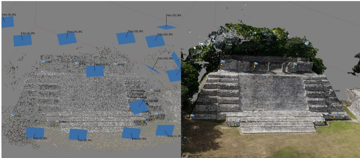
**Figure 6: Reconstruction of the image scene with sparse point cloud and positioned and oriented images (left) and the dense point cloud of the same scene (right)**
