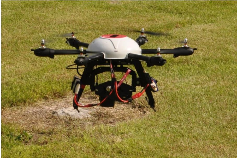
**Figure 3: Close-up of the UAV, equipped with a digital camera aiming downwards and two LiPo batteries mounted on each side of the frame**
