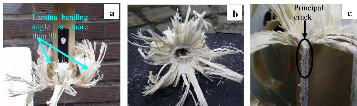
Figure 10 (a & b): Failure pattern of CP1 and CP2 series (c) Cut section of the tube
