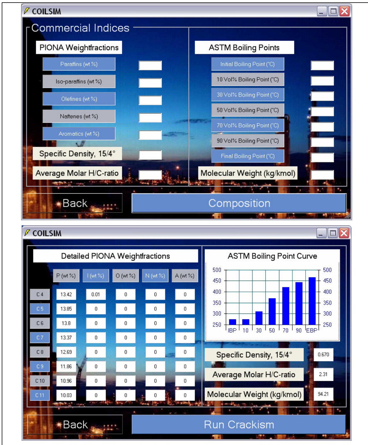
Figure 7.3: The input and results screen of the graphical user interface (GUI) for a mixture with an average molecular weight of 90 and containing only paraffinic components
