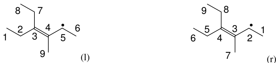
Figure 3.3: Non-unique numbering of a species (l) main chain 1 \rightarrow r ; (r) main chain r \rightarrow 1
