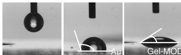
Figure 7-5: Contact angle measurements on gold and on a sensor chip, coated with gel-MOD.
