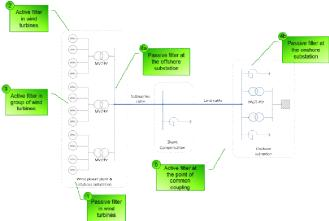
Fig. 1. Harmonic mitigation methods in wind power plants.
