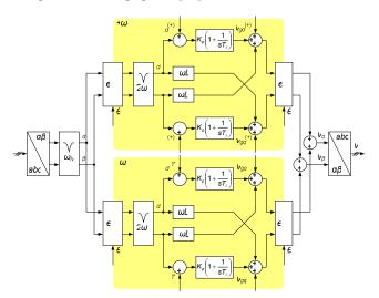
Fig. 4. Typical state-of-the-art wind turbine current control in
