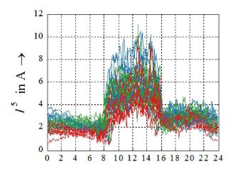
Fig. 6. Total 5<sup>th</sup> harmonic current as a function of time of day, measured at the busbar of a public LV grid with installed PV power of 332 kW
