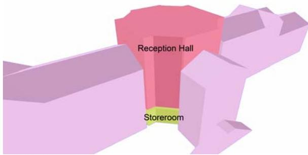
Figure 3: Each building block in the architectural information model is divided in different spaces, like for instance 'storeroom' and 'reception hall'.
