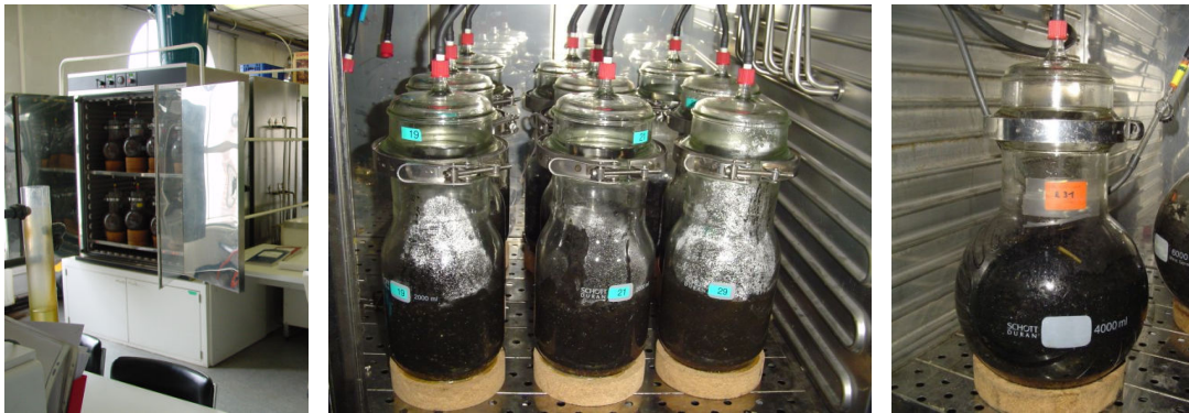
Figure 6.1. Experimental setup of batch tests for determination of biogas production potential (photo's: Peene, A., OWS, Belgium)
