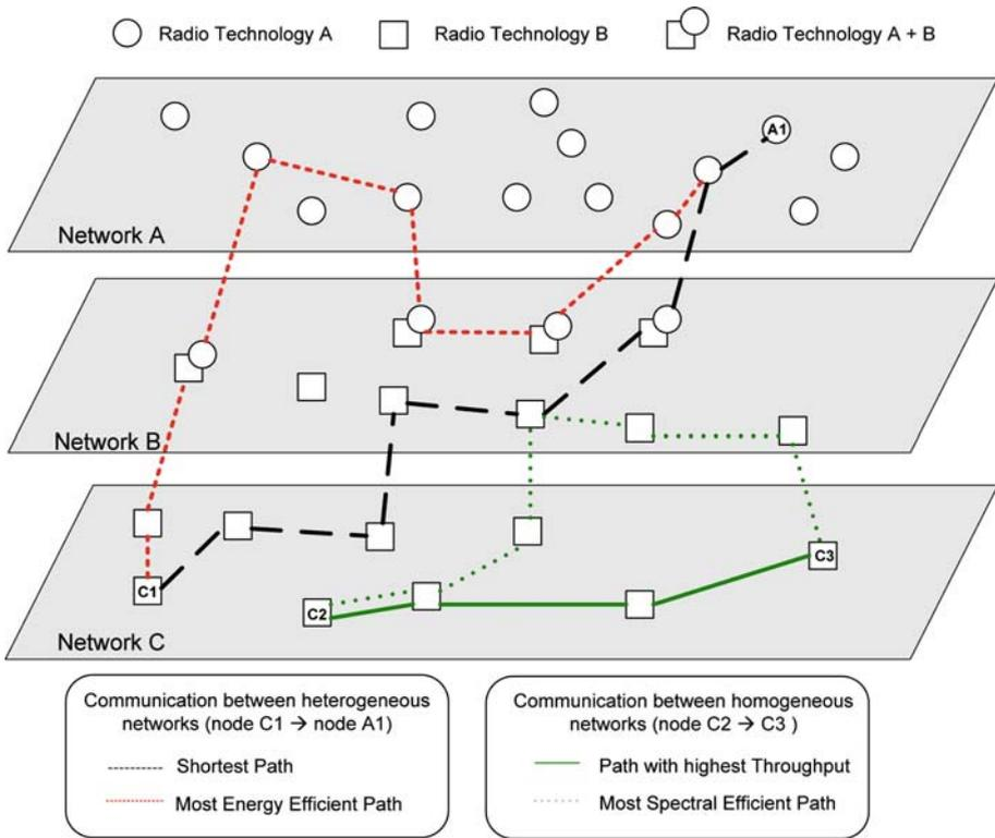
**Fig. 5** Phase 2—network binding: routing example. Two scenarios are considered. (1) Node C1 has a connection with node A1. This connection uses the multi-radio nodes of network B. The path can be optimized in number of hops or in energy efficiency (2) Node C2 communicates with node C3. The most energy efficient path uses the nodes of network B
