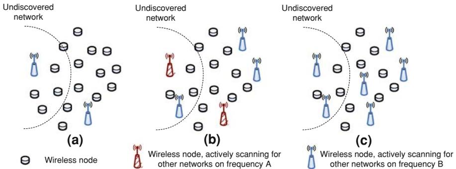
**Fig. 4** Distributed Network Discovery. **(a)** A subset of the wireless nodes is used for detecting other networks. **(b)** Other wireless nodes can be used to scan in parallel on different frequencies to ensure the timely detection of symbiotic networks. **(c)** Adding more detection nodes increase the probability of successful detection
